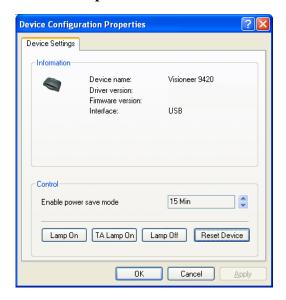
Your scanner has a built-in power saving feature that is set to power down after a period of idle time. You can set the power save mode from 1 minute to a maximum of 10 hours.
